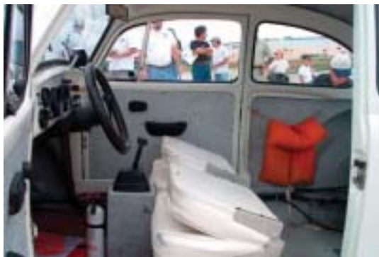
One of Creative Car Craft's most unique products is the Water Bug, a VW Beetle made entirely of fiberglass—even the wheels—that can drive on water.
