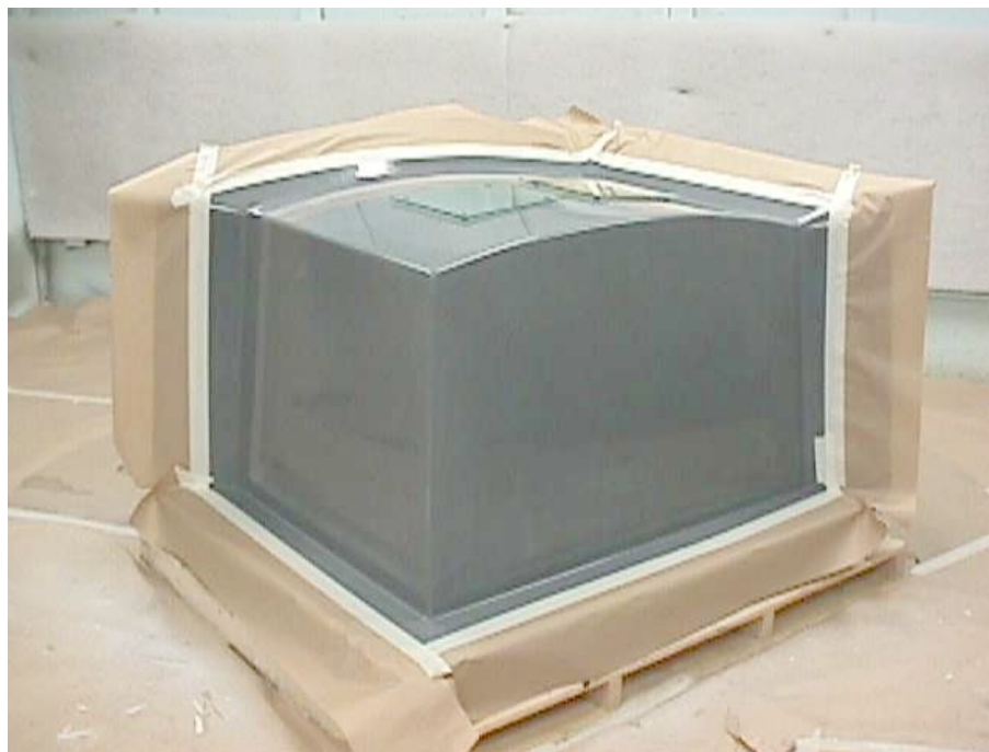
Figure 7 – Mold Flanges and Masking
