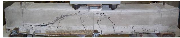
c) Shear failure of specimen 3
