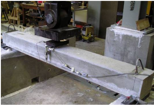
Figure-6 Experiment setup of specimen 4 prior to loading
