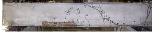
b) Shear failure of specimen 2
