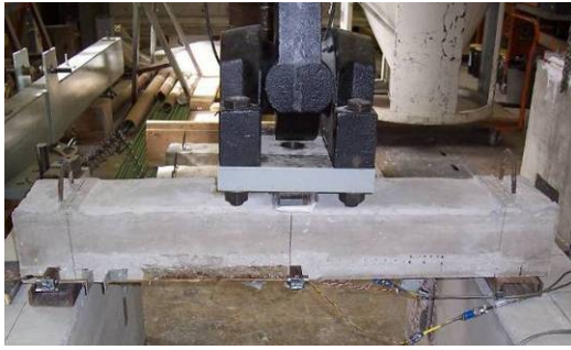
Figure-5 Experiment setup of specimen 1 prior to loading
