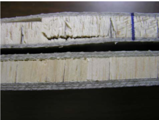
Figure 9. Failure Mode for “EGB-150” Core Material, Top: Vacuum-Infusion, Bottom: Hand Lay-up
