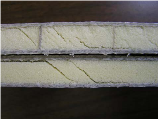
Figure 13. Failure Mode for “PURWEB-90” Core Material, Top: “W” Orientation, Bottom: “L” Orientation
