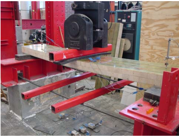
Figure – 11 Three-point bending test setup of FRP3.
