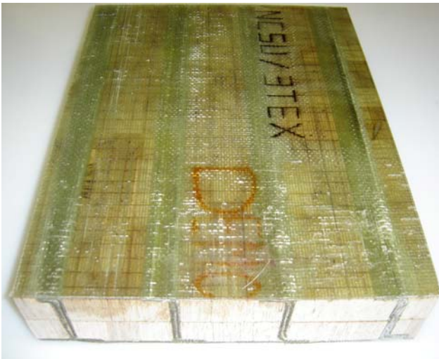
Figure – 5 Prototype 2 nd generation 3-D GFRP deck with constant cross section.
