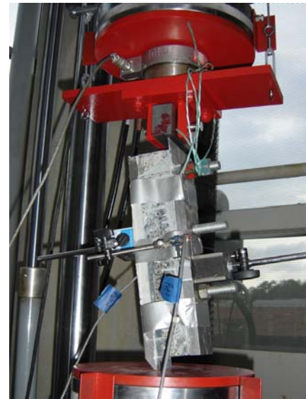
Figure – 9 Shear connector failure.
