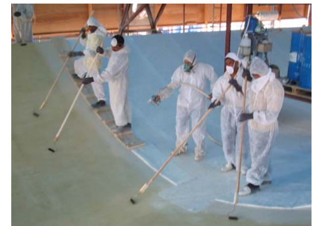
Figure 5 (a) - Manufacturing by Open Contact Mould Technique
