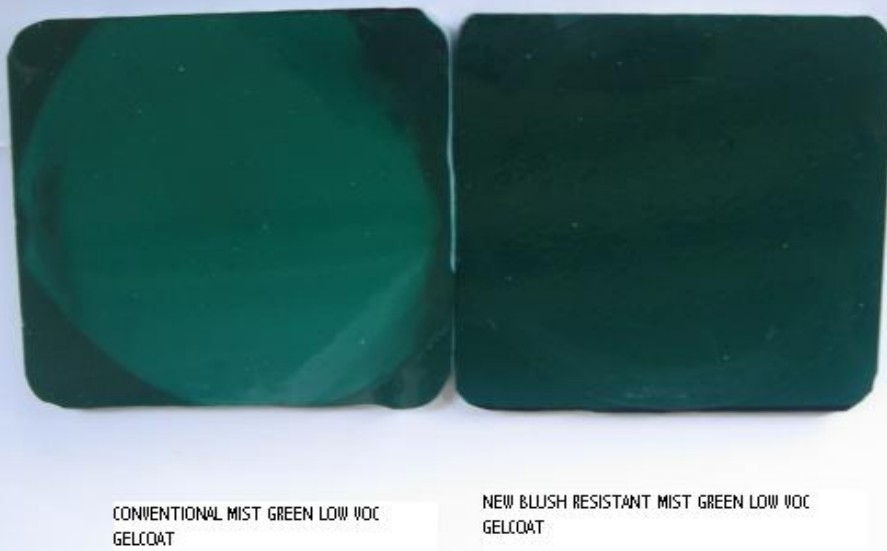
FIG 3: BLUSH TEST PANELS AFTER 100 HOURS AT 85C
