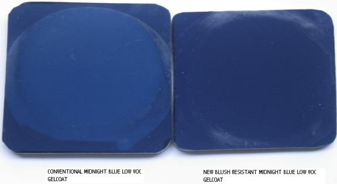
FIG 2: BLUSH TEST PANELS AFTER 100 HOURS AT 85C
