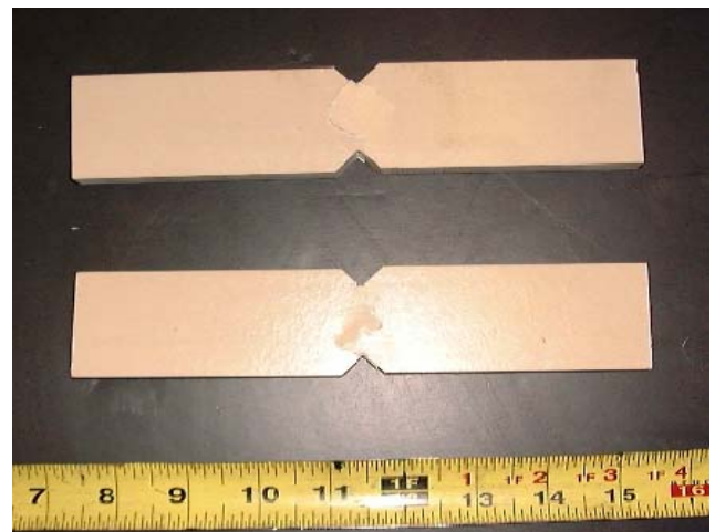
Fig. 7. A photograph of failed shear test specimen
