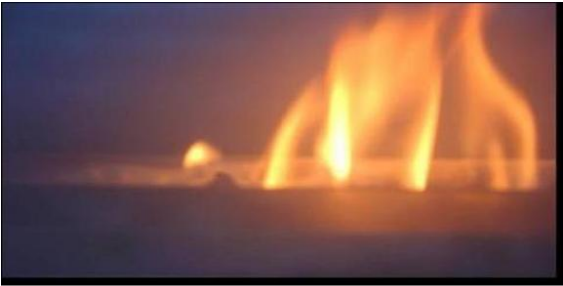
Figure 1 Burning of C20 nanocomposite film
