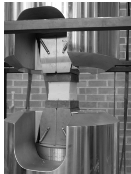
Figure – 16 Test set-up for compression specimens
