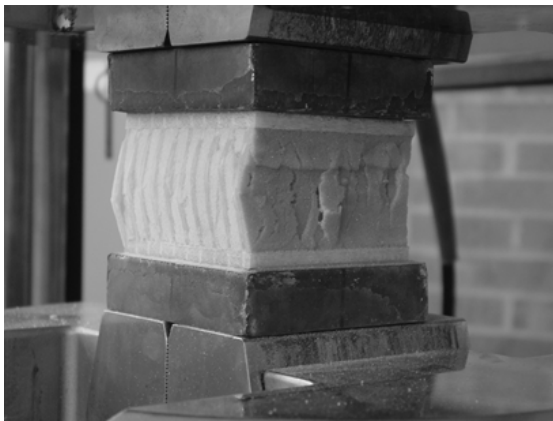
Figure – 21 Buckling of through thickness fibers at failure
