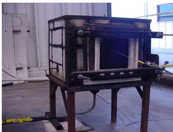
Figure 3: Small Scale Fire Test Furnace
