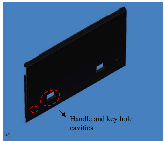
Fig. 3: Redesign of battery door to achieve a single component structure using thermoplastic composite technology (LFT)
