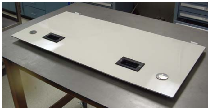
Fig. 8: Finished and painted battery box door
