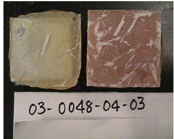
Figure - 13: Adhesive or Glue Failure: % Failure Type: Laminate = 5%, Facing = 0%, Adhesive = 95%
