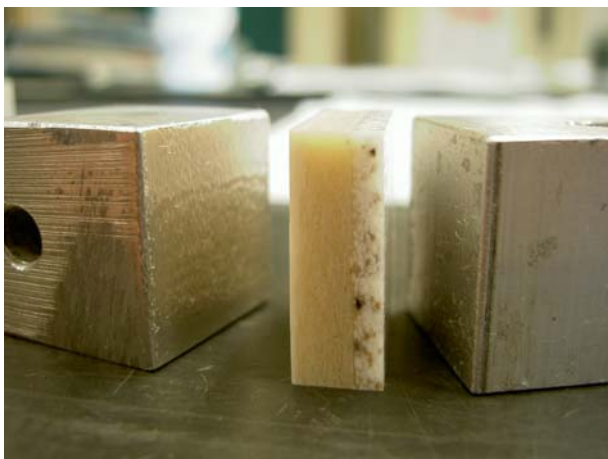
Figure - 3: A specimen and the two loading blocks ready to be bonded.
