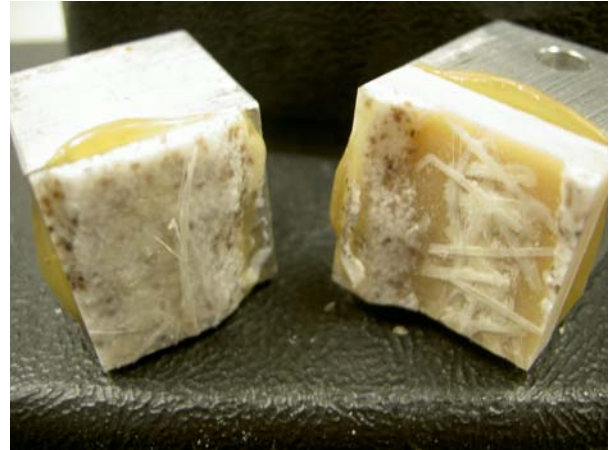
Figure - 9: Substrate or Facing Failure. % Failure Type: Laminate = 68%, Facing = 32%, Adhesive = 0%
