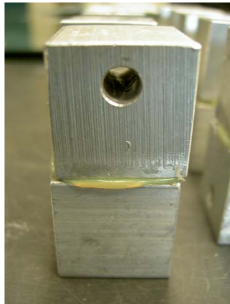
Figure - 5: Two loading blocks glued together to test glue bond strength.
