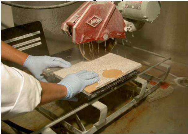
Figure - 1: Cutting a sample on the wet saw.
