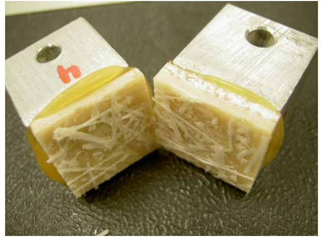
Figure - 8: Laminate or Core Failure. % Failure Type: Laminate = 100%, Facing = 0%, Adhesive = 0%
