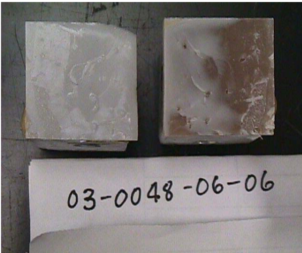
Figure - 11: Substrate or Facing Failure: % Failure Type: Laminate = 40%, Facing = 60%, Adhesive = 0%
