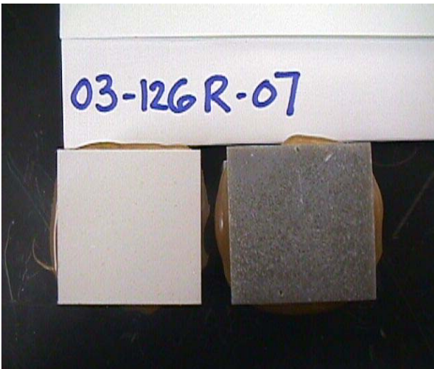
Figure - 12: Substrate or Facing Failure: % Failure Type: Laminate = 0%, Facing = 100%, Adhesive = 0%
