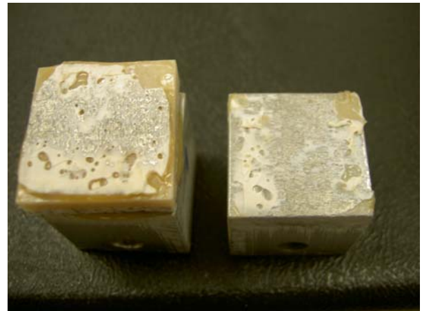
Figure - 10: Glue Failure: In this case Cohesive Failure. % Failure Type: Laminate = 5%, Facing = 0%, Adhesive = 95%
