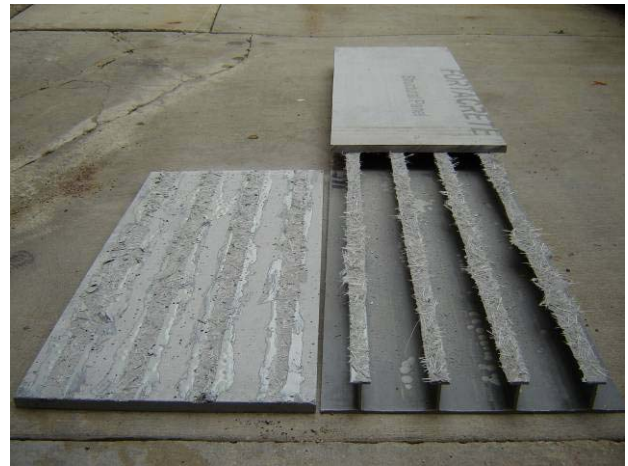
Figure – 12. Epoxy-bonded specimen cut to reveal debonding failure (Specimen 1).
