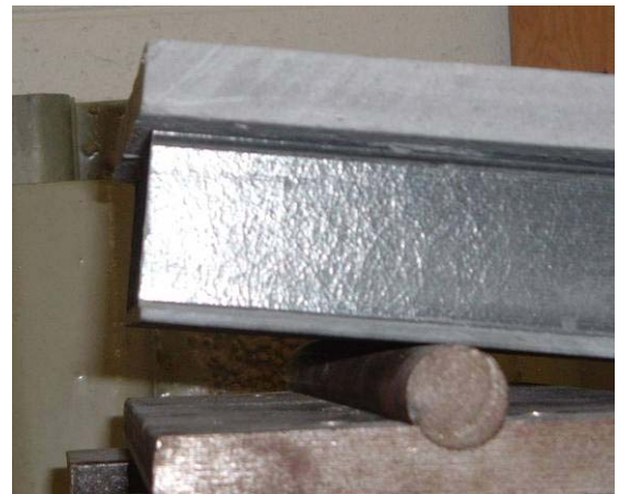
Figure – 13. Slip witnessed during gradual failure of mechanical fasteners (Specimen 2).
