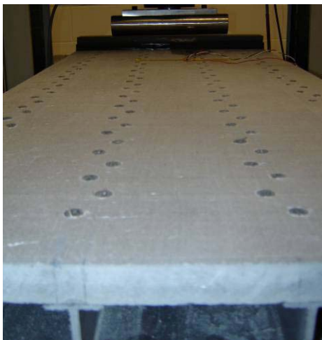
Figure – 3. Mechanically fastened cement board specimen displaying fastener layout (Specimen 3).
