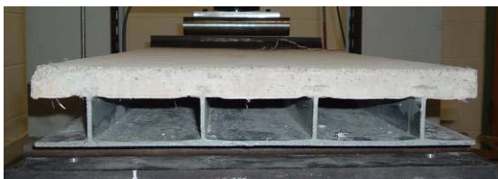
Figure – 4. Concrete specimen displaying FRP flanges embedded in concrete (Specimen 4).
