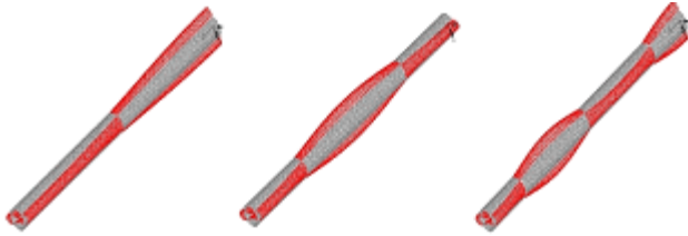
Figure – 9. Three-Dimensional Buckled Shape of Pipe
