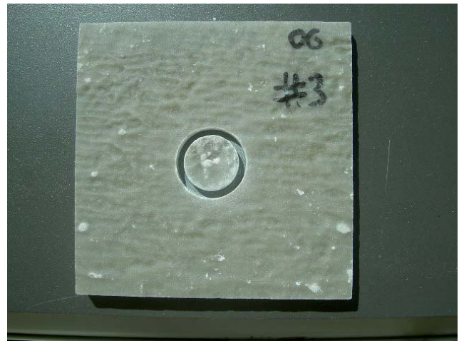
Figure - 2: The laminate side of the sample. The \frac{3}{4} in cut is roughly equal to the size of the impact plunger.
