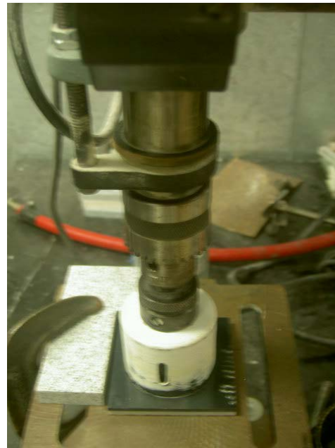
Figure - 1: Cutting a sample with a drill press.
