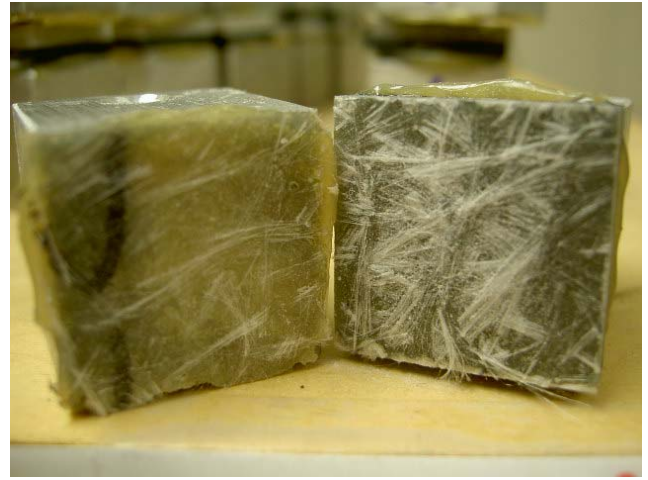
Figure -9: All of the tensile adhesion samples broke in the laminate side or adhesive, and not in the bond: just one of the many problems with this test.
