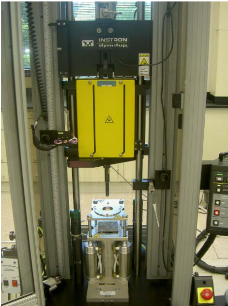
Figure - 4: The impact testing machine with the weight in the raised position.
