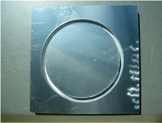
Figure - 3: The acrylic side of the sample. This side is opposite the impact.
