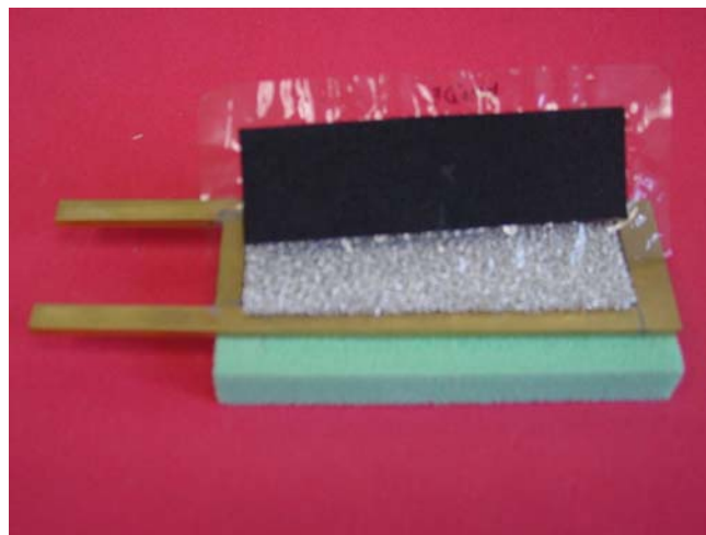
Figure – 2. Conceptual diagram of pultruded fuel cell panel.
