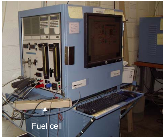
Figure – 10. Fuel cell connected to test stand.
