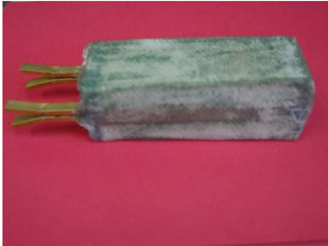
Figure – 4. Multifunctional fuel cell constructed through the VARTM process.
