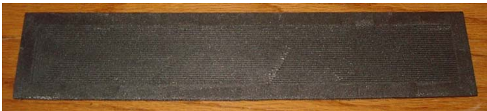
Figure – 5. Channeled composite monopolar plate (pre drilling).
