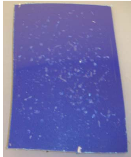
Figure 6: Heavy Marring on Chipping Resistance Test Specimens
