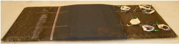
Figure - 7. Doubler-plate joint panel with embedded DSS sensors after second infusion.
