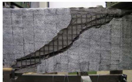
Figure 3 Concrete beams strengthen for shear with the developed MBC system. Beam loaded up to failure, see also [7]
