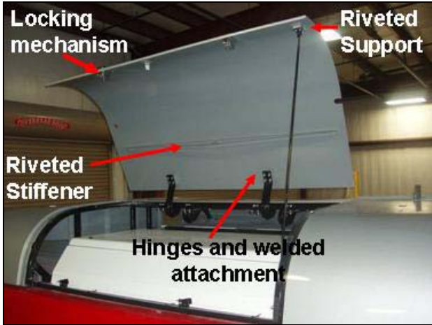
Figure – 1. AC roof cover door on a mass transit bus.
