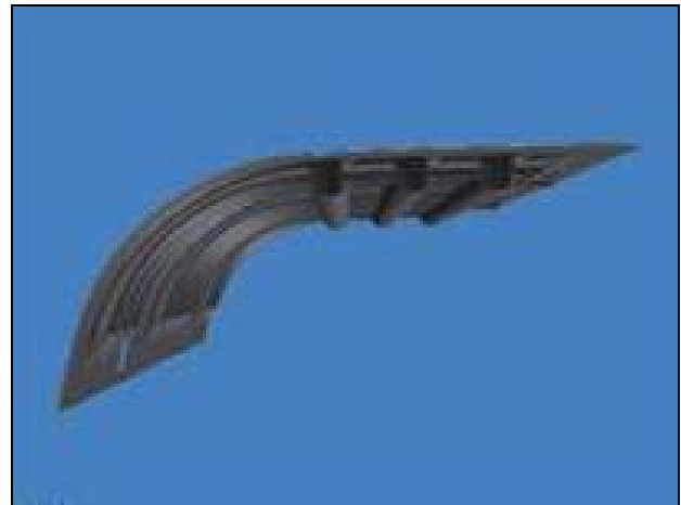
Figure – 2b. Inner rib-stiffened liner of the thermoplastic composite AC door
