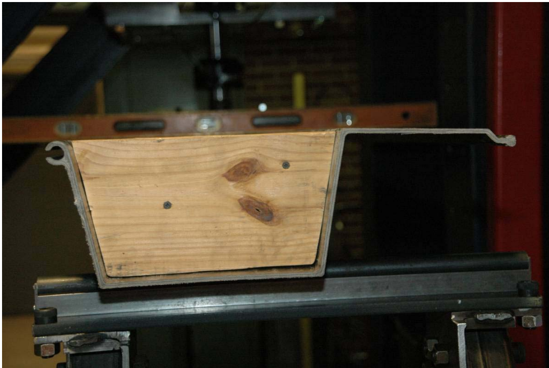
Figure 4. Wood support fit into the inside opening of the sheet piling.
