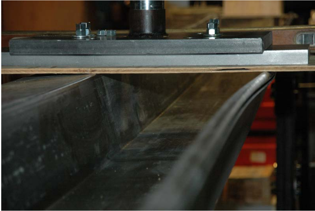
Figure 1. Buckling of unsupported sheet pile during testing at very low load levels.
