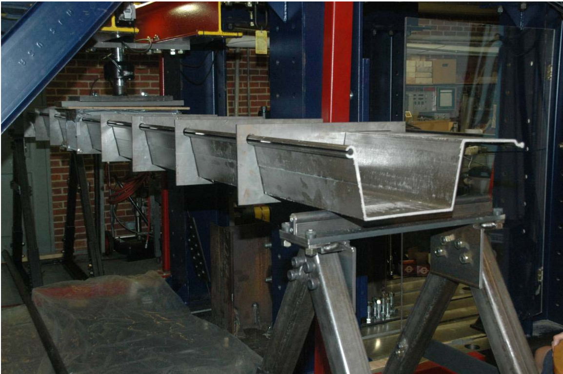
Figure 6. Flexural test setup showing the spacing of steel plates down the length of the sheet piling.
