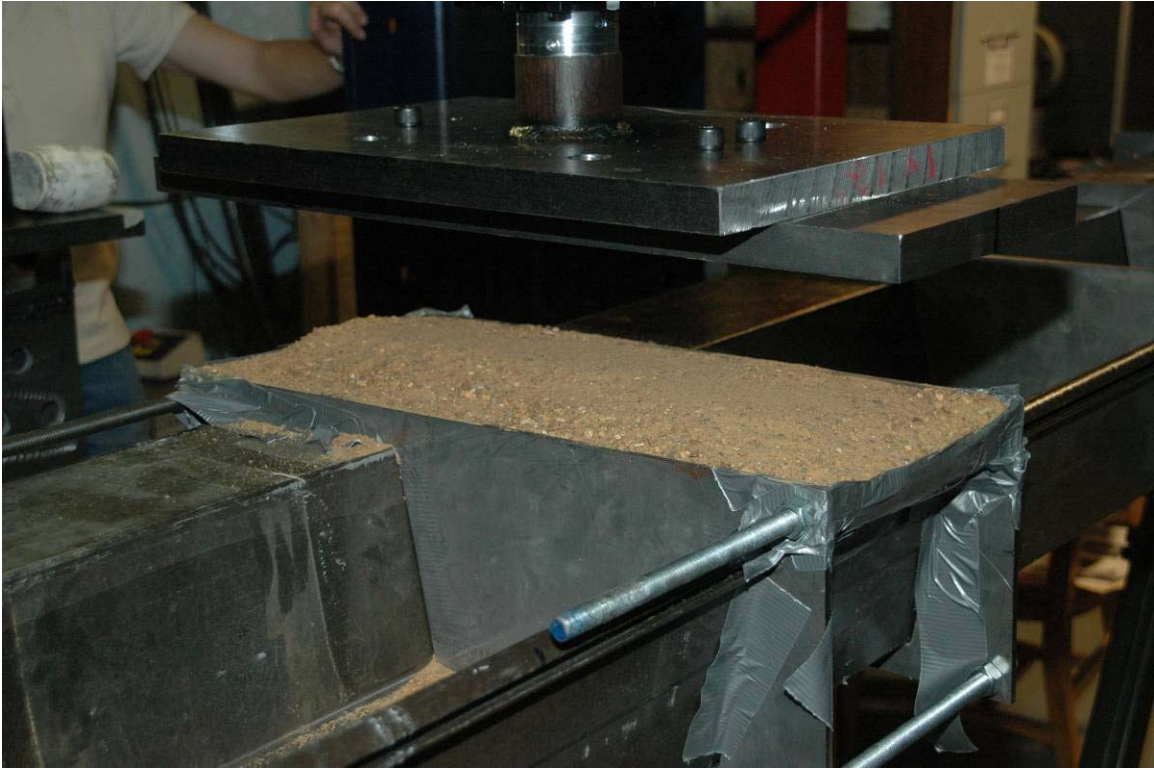
Figure 7. Steel constraint plates forming cavity filled with sand for loading of the sheet piling.
