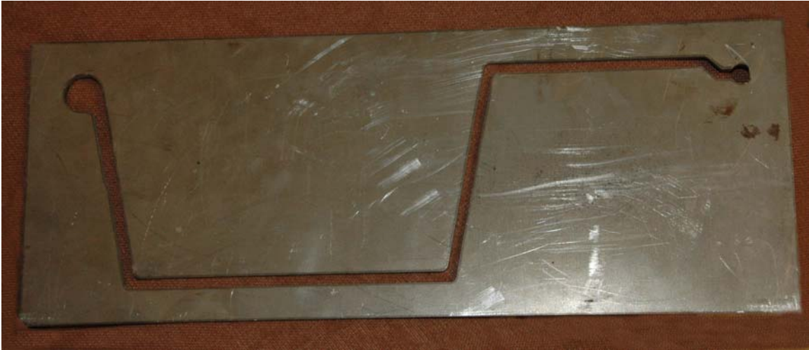
Figure 5. Steel plates showing cutout geometry.
