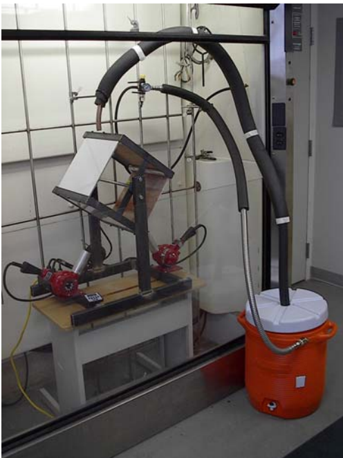
Figure – 6. Carousel Thermal Shock Test Apparatus
