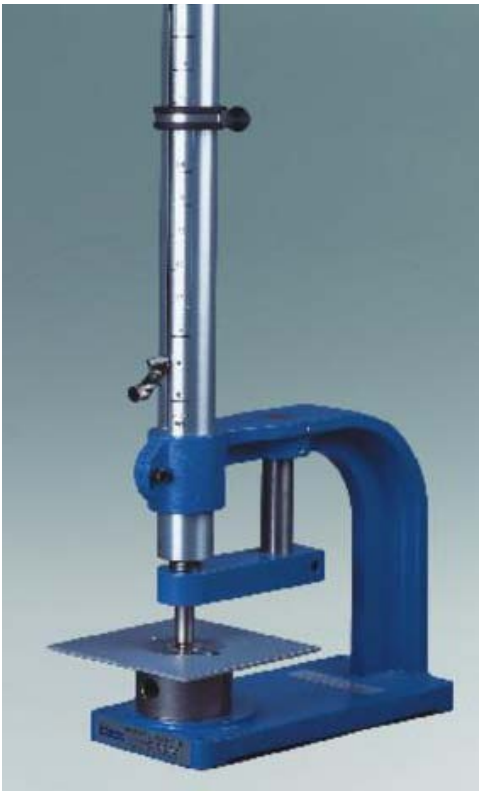
Figure – 5. Gardner Variable Height Impact Tester
